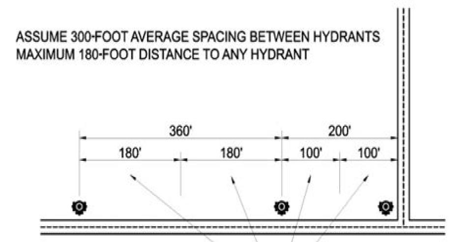
DISTANCE TO HYDRANT LESS THAN OR EQUAL TO 180 FEET - OK
